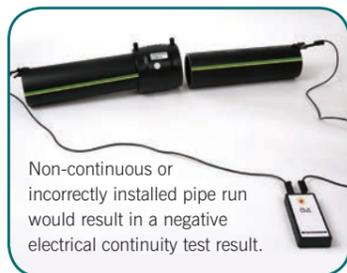
Non-continuous or incorrectly installed pipe run would result in a negative electrical continuity test result.
