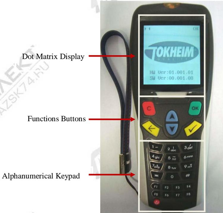
Figure 7 Main functions of Hand Held Terminal (HHT)
